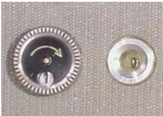
When the camera is loaded with 35mm film, you need to rotate the frame counter reset knob behind the frame counter  $\frac{1}{4}$  turn after every 10<sup>th</sup> picture. Rotating the reset knob causes the frame counter to return to 1. Otherwise, the counter will go to frame 11, 12 and then red dots with no frame spacing control. In other words, you will not get all of the pictures on your roll of 35mm film, the film will wind all of the way to the end without stopping. The
