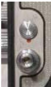
The button above the shutter release is a shutter release-locking switch, red indicates the shutter is not locked.
